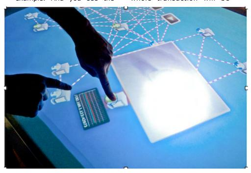
Figure 3. By touching a producer node you will see a preview of the video stream. The small graph underneath shows real-time CPU load measurements.
