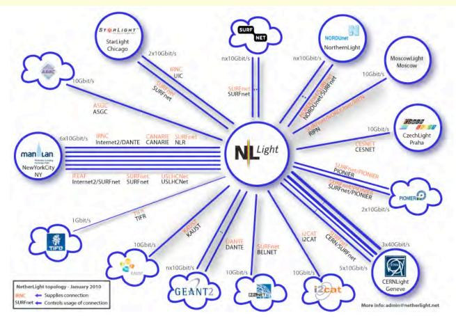
The above diagram shows the January 2010 international connectivity at NetherLight, the GLIF Open Lightpath Exchange (GOLE) in Amsterdam. All other circles in the diagram are also GOLEs like NetherLight, the clouds are the networks connected to NetherLight that are capable of supplying lightpaths. Details of all GOLEs can be found on the GLIF website under Resources: http://www.glif.is/resources/
