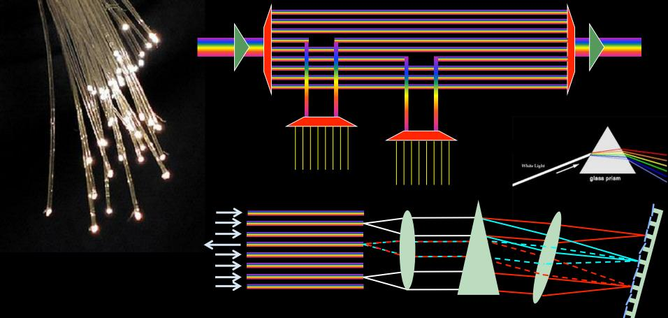
Per fiber: ~ 80-100 colors \* 50 GHz Per color: 10 - 40 - 100 Gbit/s About 10 Tbit/s per fiber long dist. BW \* Distance ~ 2\*10<sup>17</sup> bm/s Wavelength Selective Switch
