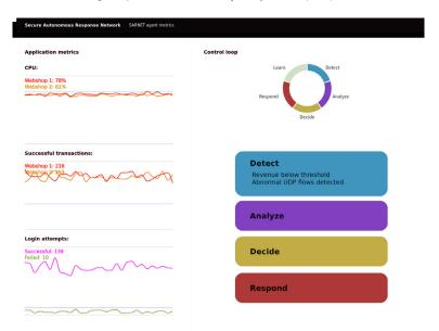
Fig. 5. Top right part of user interface of the SARNET-agent, it visualises the metrics the agent uses, the control loop and the decisions taken.
