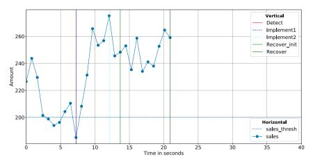
Fig. 9. Successful run with one threshold (DDoS attack). Note: The implement1 line is plotted on top of the detect line since the events occurred at the same time.
