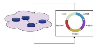
Fig. 1. The SARNET control loop.
