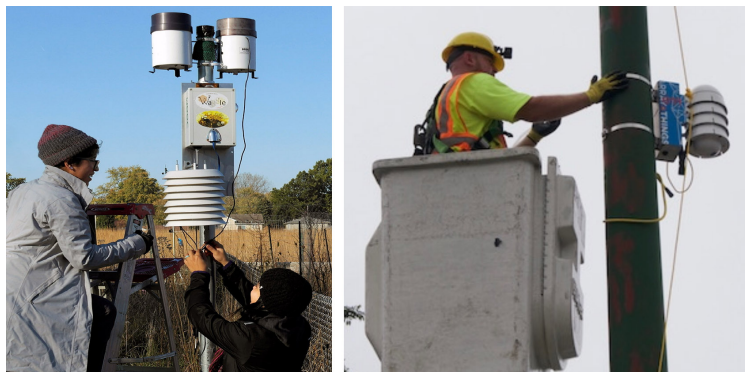
Figure 2: Left: Two Northwestern University students put up a Waggle node in a prairie to perform environmental monitoring; Right: The Chicago Department of Transportation installs an Array of Things node on a pole in the city.
